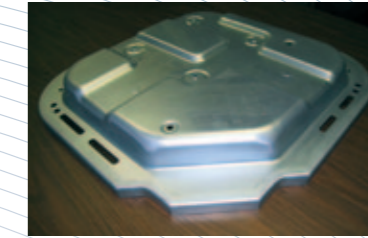
Physical part obtained right the first time based on simulation work Courtesy: Doerfer Companies
